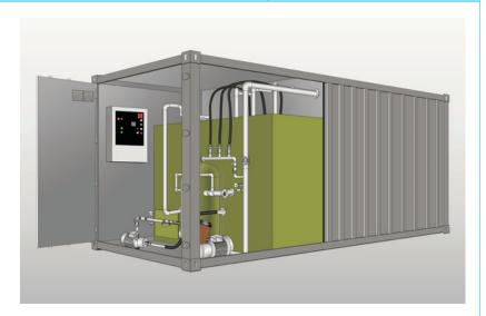
Facet's SMS Sewage Modular Systems for inland applications have been designed for gravity or pumping treatment of domestic sewage, and built to be installed above ground. These systems carry out the sewage treatment by biological means. These are of the active sludge, aerobic and extended aeration type, without requiring any other kind of dosing or additivation.
